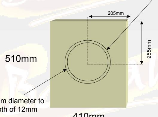
306mm diameter to depth of 12mm
