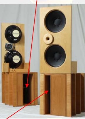
Screw 18inch driver from this side so the metal frame is visible through the front vent
